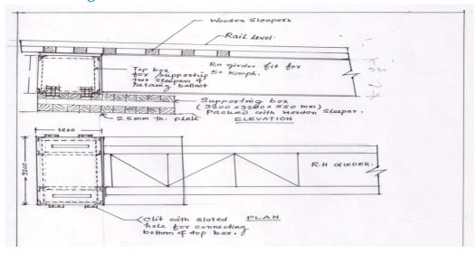
The drawing to be followed is "Temporary support of Box Crib for relieving girders for length upto 20.40 m" having drawing no PCE-24019-HQ-TP-2016.
