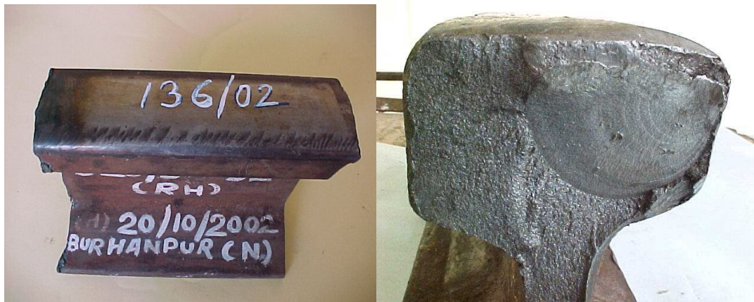
Figure 7 (a) & (b) : Showing Gauge Checking Cracks and subsequent Fatigue Fracture
