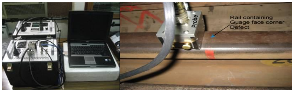
Plate 6: Power Box Set up from Innerspec and Testing of Rail Containing Natural GFC defect
