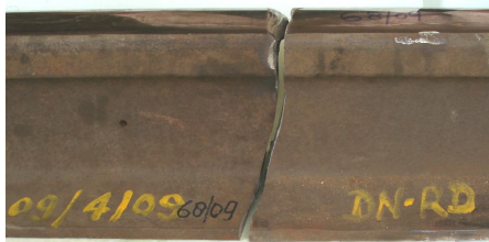
Plate 3: Rail pieces in juxtaposition exhibiting angle of inclination (Approximately 6 degree from vertical) of Transverse Defect. Ultrasonic test report of the rail less than 15 days prior to failure did not indicate any defect. Question: Did orientation play a role in non detection?
