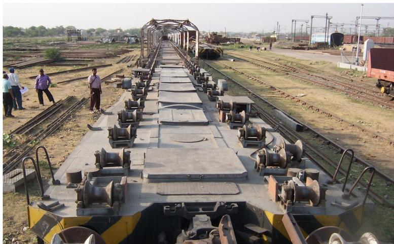
yard and loaded on this machines in four layers. In fact a bundle of four track panel is loaded on every special BRH. On such BRH special rollers are provided on which the bundles of panels are moved longitudinally by pulling mechanism. By such pulling action, bundles of panels are brought within the reach of gantry.
