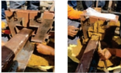
Fig.1.7 Luting of the mould
