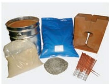
Fig. 2.3 (a) Portion, Luting sand, Crucible, mould & Igniter
