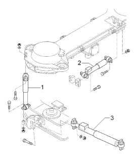
1. Vertical damper 2. Lateral damper 3. Yaw damper
