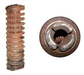
Fig. 6.6 Spring Loaded Friction Snubber
