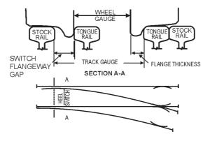
Fig. 3.4 Switch Flange-way gap
