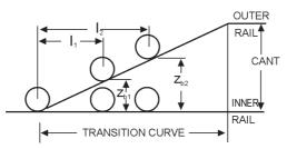
Fig.1.47 Effect of rigid wheel-base on transition curve
