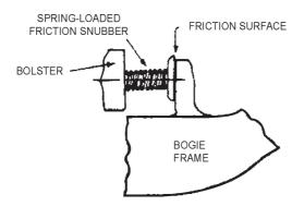
Fig. 3.35 Friction snubber arrangement
