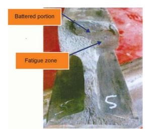
Fig. 9.2 Fractured rail face
