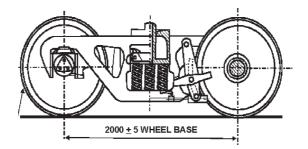
Fig.1.33 : Rigid wheel base, I, in case of a bogie stock
