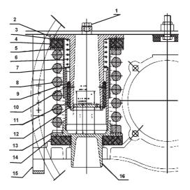
1.Screw with sealing washer 2. Guide 3. Protective tube 4. Rubber washer 5. Top spring seat 6. Dust shield spring 7. Dust shield 8. Spring 9. Guide ring 10. Rubber packing ring 11. Guide bush 12. Circlip 13. Compensating ring 14. Rubber washer 15. Safety strap 16. Lower spring seat
