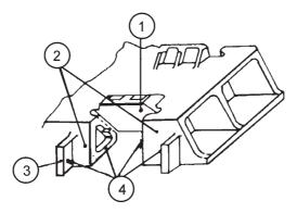
Bolster pocket slope surface liner 2. Bolster land surfaces
