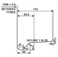
Fig. 6.3 Thick IRS Tyre Profiles for BG Loco
