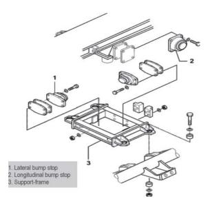
Fig. 5.28 Bump Stop Arrangement
