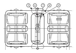
1.Axle box spring 2. Bolster spring 3.Swing link 4. Spring plank 5. Bolster 6. Side bearer 7. Centre pivot 8. Bogie frame 9. Anchor link
