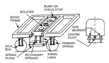
**Fig.** 5.1 illustrates the schematic arrangement of such a suspension.
