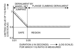
Figure 1.20 Limiting values of Y/Q ratio vs time duration
