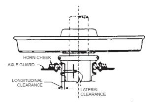
Fig. 3.26 Lateral and longitudinal clearances (plan)
