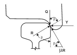
Fig.1.14. Forces at rail-wheel contact with positive angularity
