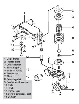
Fig. 5.19 Components of Primary Suspension
