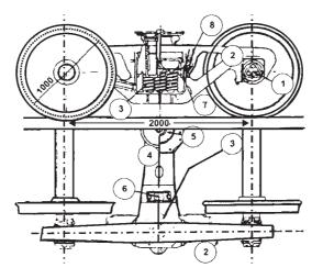
Roller bearing axle box 2. Side frames 3. Main bearing helical spring nest 4. Bolster (with guide lugs) 5. Centre pivot
