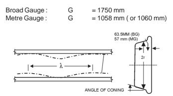
Fig.1.29 : Kinematic oscillation of a wheelset
