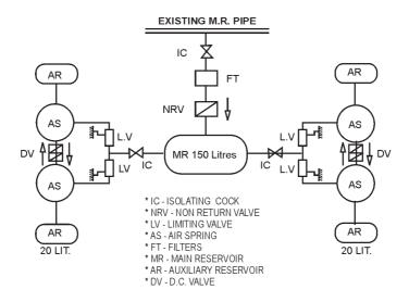
Fig. 3.33 Air spring system
