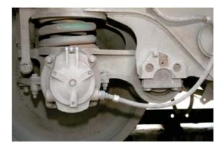
Fig. 5.18 Primary Suspension Arrangement
