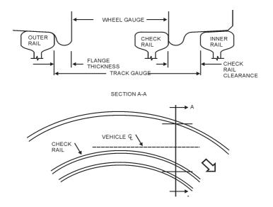
Fig. 7.5 Check rail on curve
