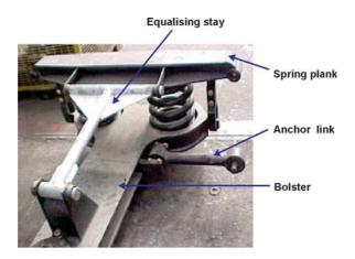
Figure 5.8 Equalising Stay Arrangement
