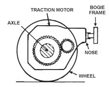
Fig. 6.1 Axle hung nose suspended traction motor
