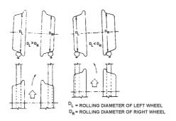
Figure 1.24 wheelset guidance by tread conicity
