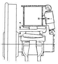
Figure 6.24 Bump Stop Clearances at primary stage
