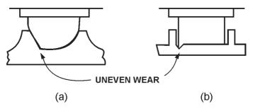
Fig.3.40 Uneven wear in (a) hemispherical pivot, (b) flat pivot
