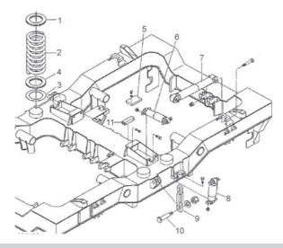
1.Insulating bases top 2.Coil spring 3.Compensating plate 4.Insulating base bottom 5.Vertical bump stop 6.Lateral hydraulic damper 7. Yaw hydraulic damper 8.Vertical hydraulic damper 9.Safety chain 10. Pin 11. Lateral bump stop
