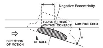
Figure 1.7 Negative angularity (Plan)
