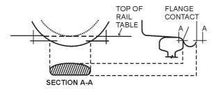
Figure 1.4 Sectional plan of wheel flange at the level of flange-to-rail contact
