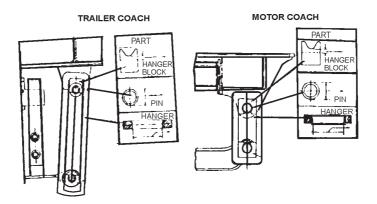
Fig.5.15 Hanger and Hanger block
