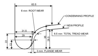
Fig. 3.13 Condemning wear limit
