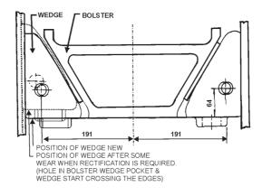
Fig. 4.10 (a) Friction Snubber Wedge Arrangement
