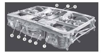
Fig. 5.2 ICF All-coil Bogie
