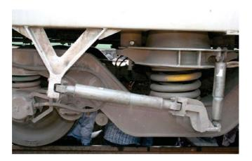
Figure 5.21 Secondary Suspension
