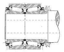
Fig. 3.23 Tapered cartridge roller bearing
