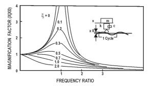
Figure 1.36 Magnification factor for a simple spring-mass damper system
