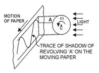
Fig.1.27 Representation of sinusoidal motion
