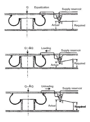
Fig. 3.34 Air Spring control mechanism
