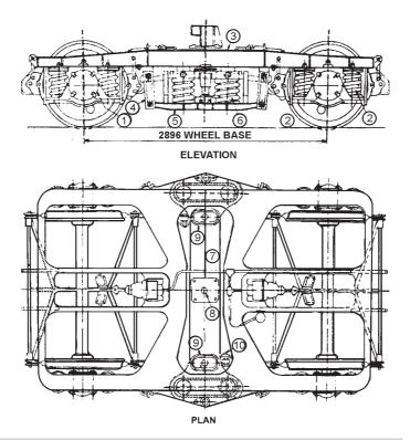
1. Wing Type Roller Bearing Axle Box 2. Primary Springs (helical) with dashpots inside 3. Bogie Frame 4. Swing Links 5. Spring Plank 6. Secondary Springs (helical) 7. Bolster 8. Centre Pivot 9. Side Bearers 10. Anchor Link
