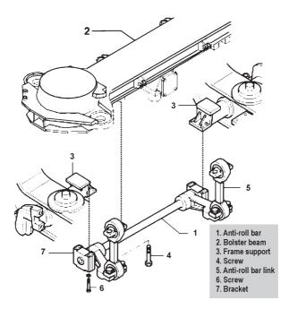
Figure 5.25 Anti – roll Bar Arrangement
