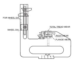
Wear measurement gauge is as shown in figure 3.12.
