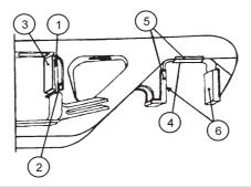
1. Side frame column sides 2. Anti-rotation lugs 3. Side frame friction liners 4. Pedestal crown roof 5. Pedestal crown side and pedestal sides 6. Pedestal jaw
