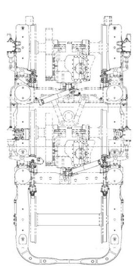
Fig. 6.14 (a) HTSC bogie – General arrangement
