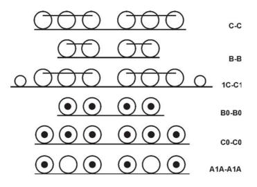
Fig. 6.2 Axle and Traction Arrangement
