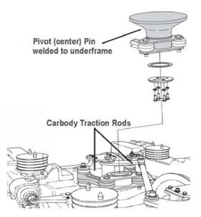
Fig. 6.17. Car Body Pivot Pin and Socket arrangement
