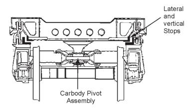
Fig. 6.16.Lateral and Vertical Stops
