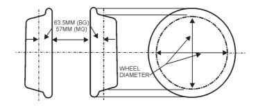
Fig. 3.19 Measurement of wheel tread diameter
