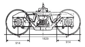
Fig. 4.4 Suspension arrangement of Talbot bogie
