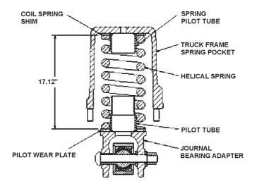
Fig. 6.18. Coil Spring Seat
