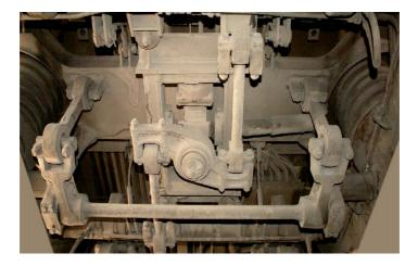
Fig. 5.26 Anti-roll Bar and Traction Centre
