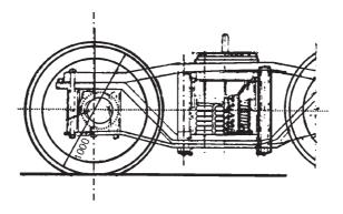
Fig. 4.5 Suspension arrangement RDSO Soft Ride bogie
