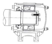
Fig. 3.22 Spherical roller bearing
