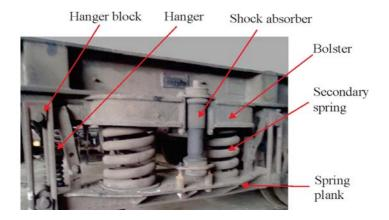
Fig. 5.4 ICF All-coil Bogie – Secondary suspension
