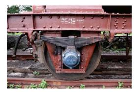
Fig. 3.25 Suspension system of 4-wheeler.
