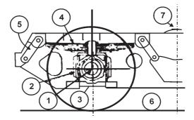
1.Roller bearing axle box 2. Horn Cheek 3.Briddle bar 4. Laminated spring 5.Shackle (Link) 6. Bogie frame 7. Centre pivot
