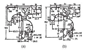
Fig.3.2 Tyres defect gauge (a) B.G. (b) M.G.
