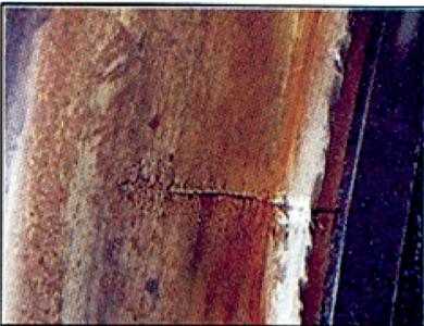
**Fig: 32 Thermal crack on tread**
