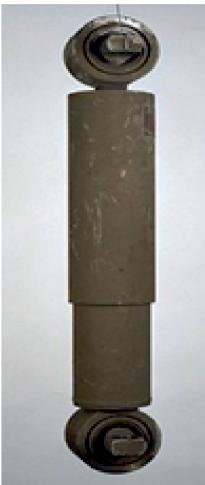
For a long service life, it is necessary for the rod oil seal to remain lubricated. The continuous inward and outward movement of the piston rod may cause oil “sweat” from the rod oil seal.
