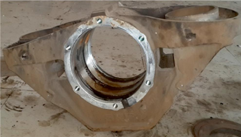
Fig 16 : Axle bearing housing photo graph
