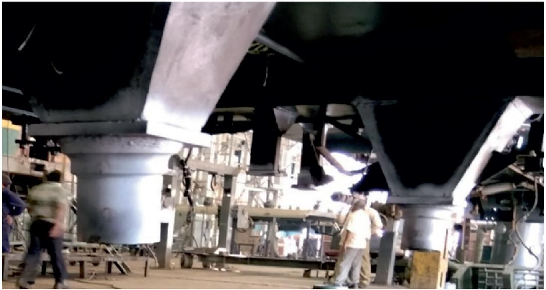
**Fig 60 : Locomotive Pivot points for connections of both bogie traction links.**
