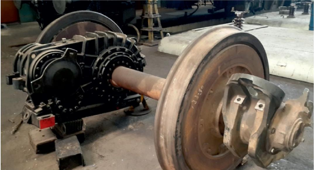
**Fig 19 : Photo of assembled wheel showing hurth coupling gear case, Axle box and brake disc**
