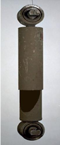
Normal contamination caused by the operating environment of the dampers is harmless.
