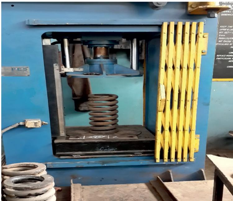
**Fig 38 : Spring deflection testing machine**
