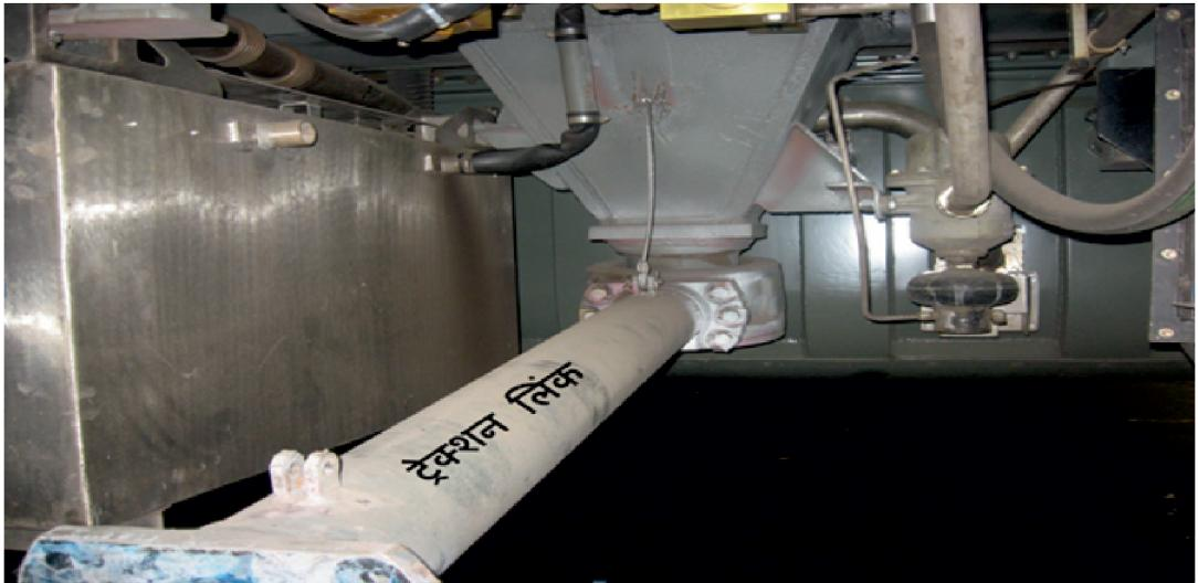
**Fig 59 : Traction link connection at loco pivot point.**
