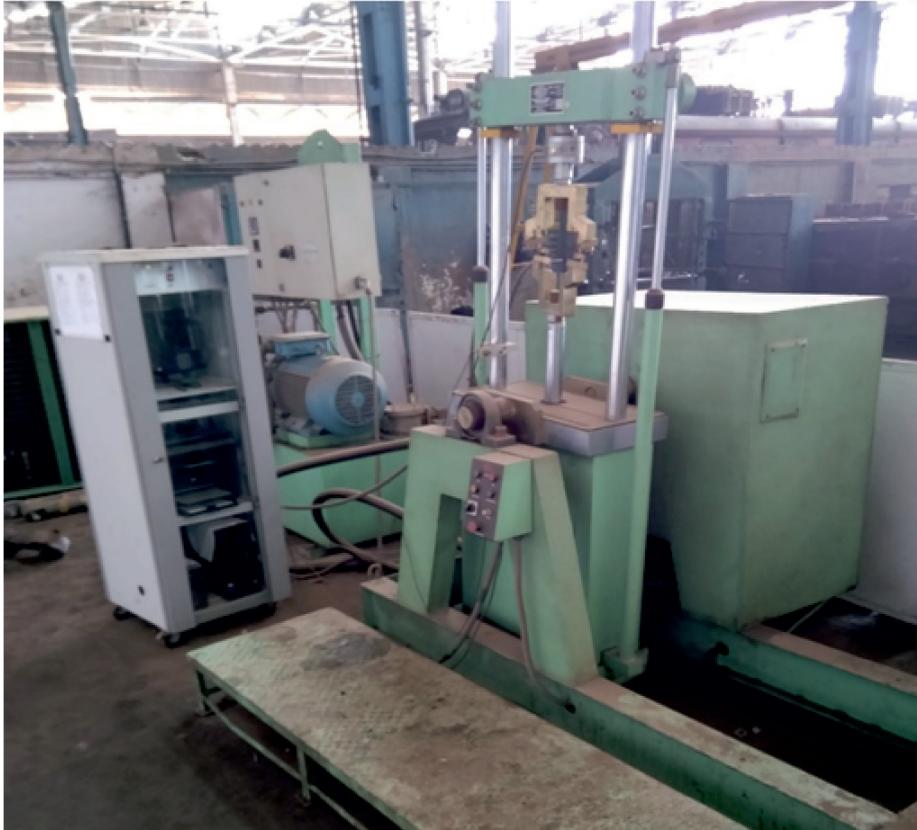
**Fig 50 : Hydraulic damper testing machine**
