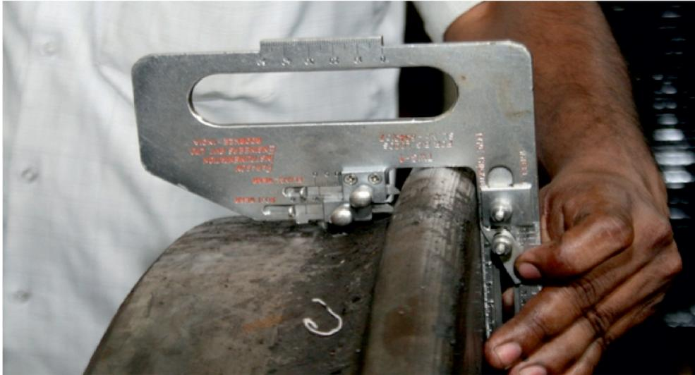
**Fig 25 : Procedure for checking wheel tread wear**
