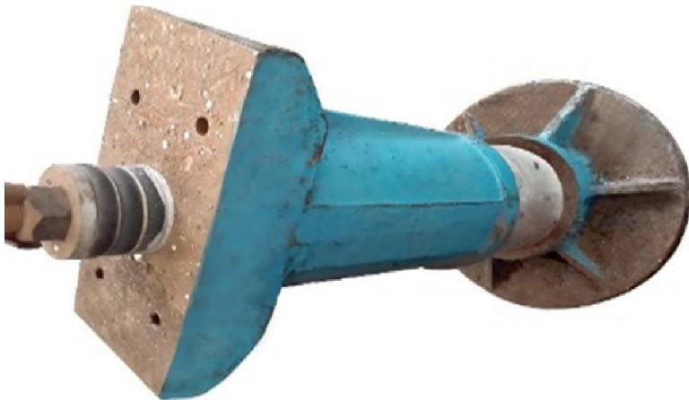
**Fig 64 : New type of buffer**
