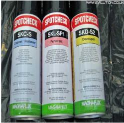
**Fig. 1: Surface Cleanser, Developer and Penetrant**
