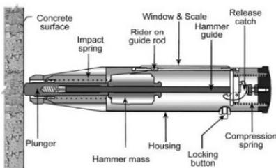
**Fig. 2: Schematic of Rebound Hammer**
