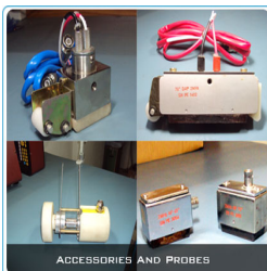
Fig. 5: Angle probe for checking of probe index and probe angle
