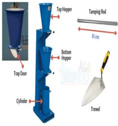
**Fig. 2: Compaction Factor Apparatus with Allied Tools**
