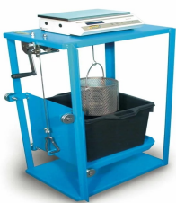
Fig. 2: Setup of Specific Gravity Test (To be used for Aggregate > 6.3 mm)
