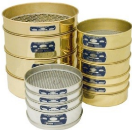
Fig. 2: Sieve (12.5 mm, 10.0 mm and 2.36 mm)
