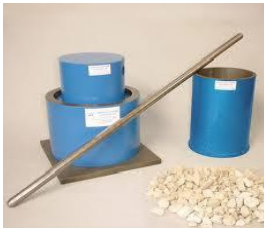
Fig. 3: Mould, Measuring Cylinder with Plunger
