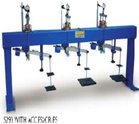
**Fig. 1: Consolidation Test Apparatus**
