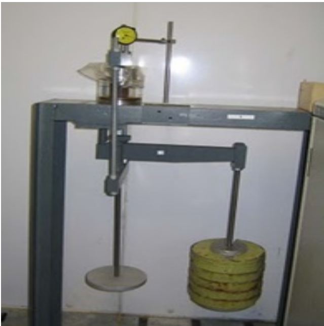
Fig. 1: Swell Pressure Test by Consolidometer
