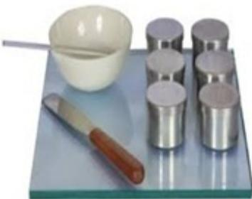
**Fig. 1: Glass Plate, Palette knives, Air Tight Containers, Spatula, Brass Rod & Porcelain Evaporating Dish**
