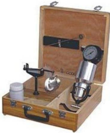
**Fig. 1: Setup for Rapid Moisture content Determination**
