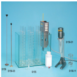
Fig. 2: Laboratory setup for Hydrometer Test
