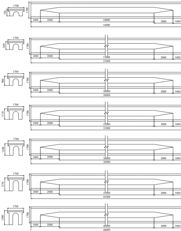
Fig.9 : Proposed cross-section and bottom view of TT-girders of span varying from 15m to 45m (symmetrical dimensions in plan are avoided).
