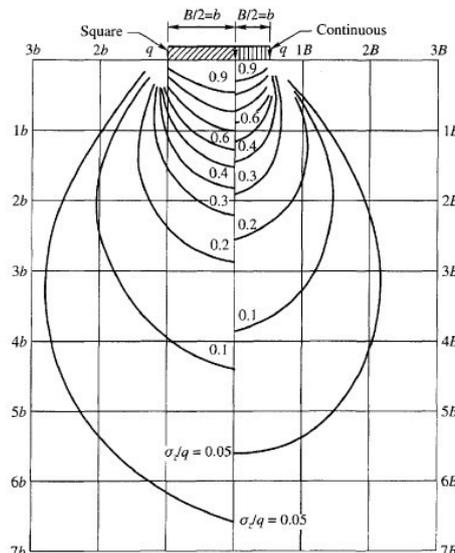
**Fig:** Pressure isobars based on Boussinesq equation for square and continuous footings
