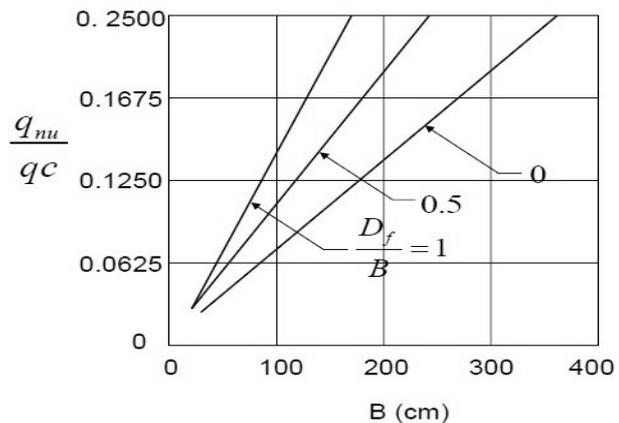
The static cone resistance,  $q_c(\text{kg/cm}^2)$  is used to determine the bearing capacity factor,  $N_\gamma$  from the correlation given by Schmertmann (1975),
