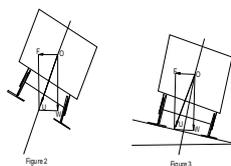
The resultant U is central for a combination of cant of track and speed of vehicle. At this equilibrium, the load carried by each wheel is the same, the springs are supposed to be equally compressed and passenger does not tend to lean in either direction.
