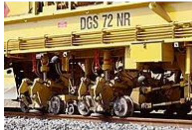
close up of the stabilization unit
