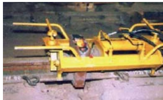
Fig. 4.7: Trimming operation by hydraulic weld trimmer
