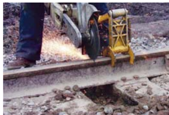
Fig. 4.1: Abrasive disc cutter
