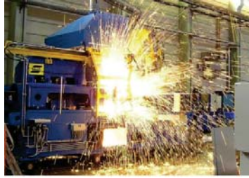
Fig. 3.1 : Welding by stationary flash butt welding plant
