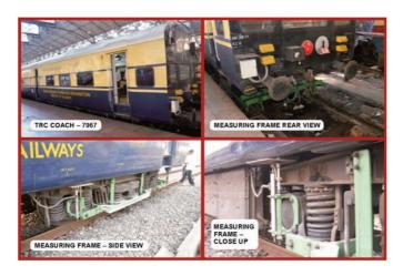
ii. With contactless laser based sensors; having LASER based contactless sensors mounted on a sensor beam welded on the rear bogie of TRC; as seen in sketch below.
