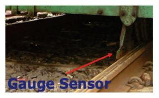
(ii) The Carbide tips are provided on the contact surfaces to reduce the wear of the sensors. (See photo along side)
