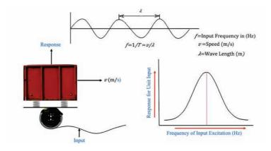
15.2 The vehicle accelerations under such circumstances chiefly depends on frequency response of the vehicle, its speed and the wavelength of the irregularity responsible for input excitations as described below:
