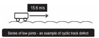
The frequency, of vibration induced, will thus be 1.2 cycles/second (=15.6/13). The natural frequency of vibration of a typical ICF coach being 1.2 Hz., it would resonate and experience wild movements at this speed (i.e. 56 km/h).
