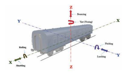
9.3. Amongst these the important parasitic movements with which a track maintenance engineer is usually concerned are lurching, bouncing and rolling and causes unwanted accelerations. Here the basis assumption is that there is no abnormality in operations and/or defect in the rolling stock i.e. being a perfect rolling stock.
