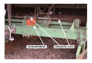
(c) Based on the sampling distance, of 25 cm, between two successive samples, for a block of 200 m length, there would be 800 readings of alignment for each rail gets recorded.
