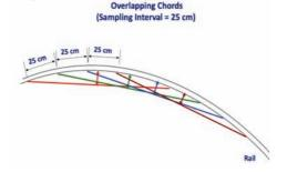
Similar principle is used to calculate twist for which the overlapping sliding base length is used.
