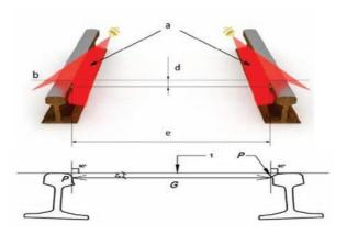
(ii) Based on the sampling distance, of 25 cm, between two successive samples, for a block of 200 m length, there would be 800 readings of gauge gets recorded.
