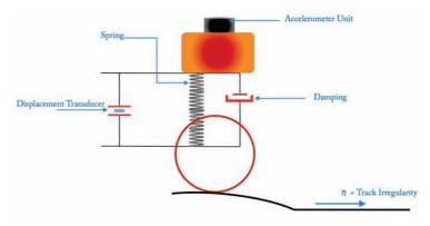
Both types of TRCs are based on inertial principle of track measurements and it is possible to have discrete values of track geometry parameters on selected sampling interval, under loaded condition on two user selectable chords in the range of 2 to 20 meter.
