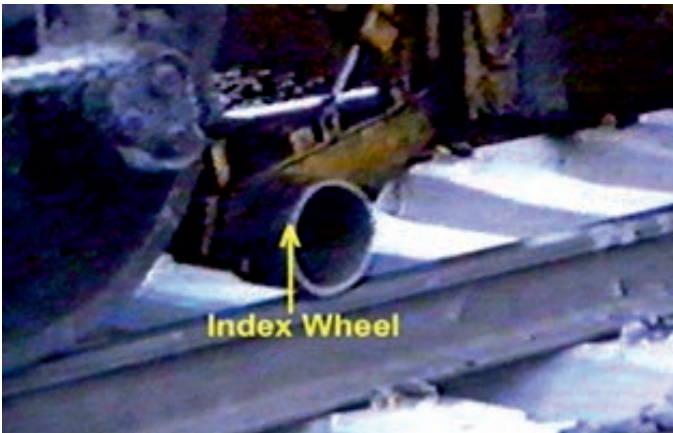
Fig. 5.10 Index Wheel for Maintaining Sleeper Spacing
