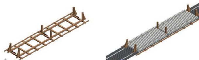
Fig. 7.1 Subframe consisting of Roller at Bottom for Rails and Sleepers on Support over it.
