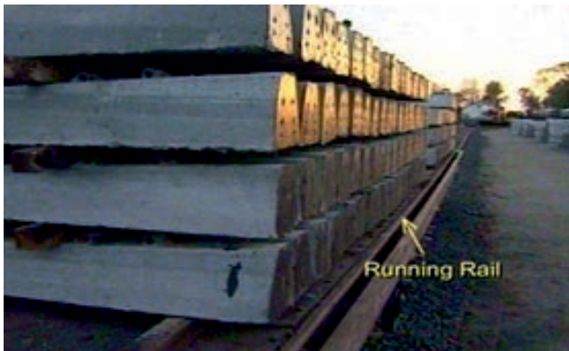
Fig. 5.12 Sleeper loaded on TRT Wagon with Spacers.
