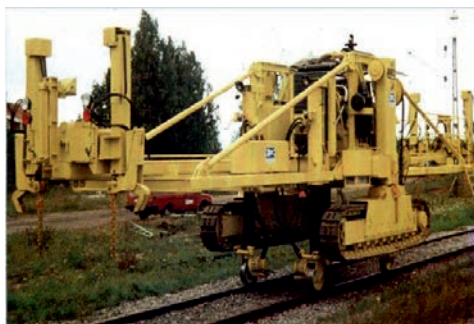
Fig. 6.3 T-28 Portal Crane on Rail
