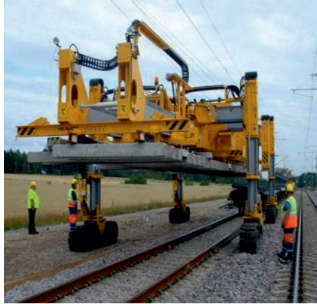
Fig. 10.3. Dessec Make Portal for Laying Fabricated Panel It does not require Auxillary track and moves on crawler.
