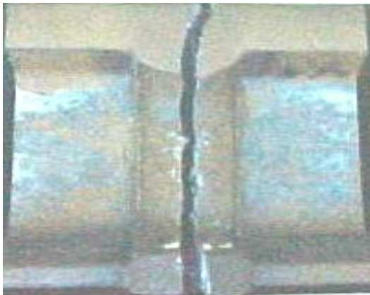
FIG. 50 : 411 - WELDING, FLASH BUTT JOINT, TRANSVERSE CRACK
