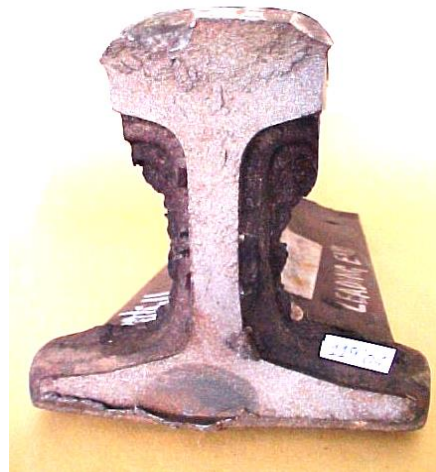
FIG. 51 : 421 - WELDING, THERMIT JOINT TRANSVERSE CRACK
