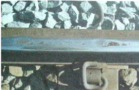
FIG. 40 : 2252 - HEAD SURFACE, WHEEL BURN REPEATED
