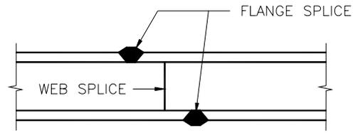
AVOIDING ACCUMULATION OF WELD JOINTS
