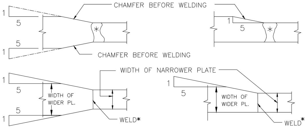
TRANSITION BY CHAMFERING THICKER OR WIDER PART
