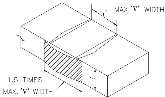
BUTT WELD END REINFORCEMENT
