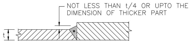
BUTT WELD WHERE TRANSITIONING IS NOT PRACTICABLE
