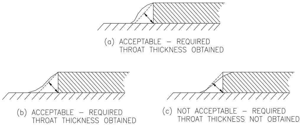
FILLET WELD EQUAL TO THE SIZE OF PLATE OR SECTION
