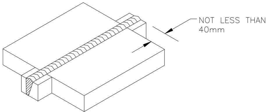
BUTT WELDED JOINT WITH RUN-ON AND RUN-OFF PLATES
