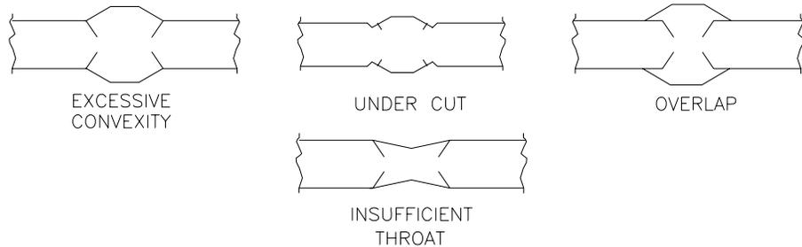
DEFECTIVE BUTT WELD PROFILES
