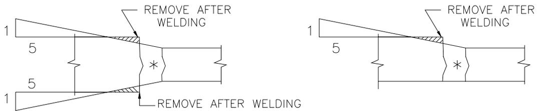
TRANSITION BY SLOPING WELD SURFACE AND CHAMFERING
