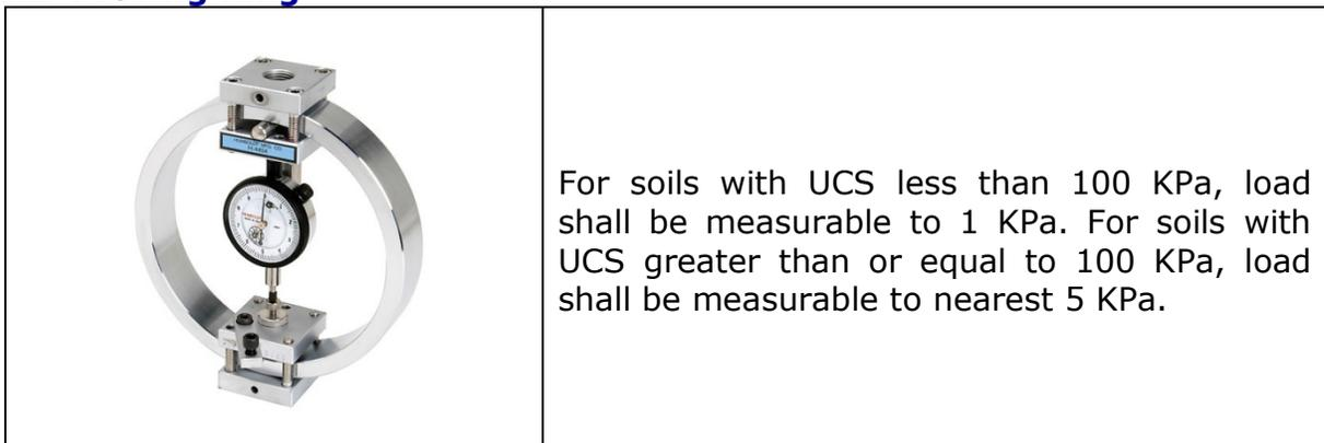
**2.3 Deformation Dial Gauge**, having a least count of 0.01mm and travel to permit not less than 20 percent axial strain.
