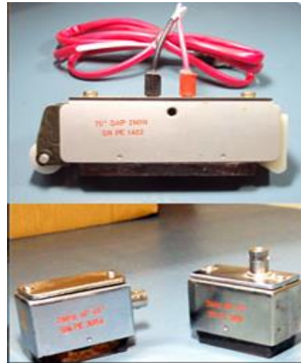
Fig. 5: Angle probe for checking of probe index and probe angle
