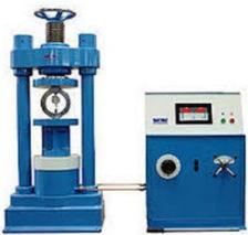
**Fig. 4: Compression Testing Machine**
