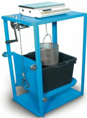
Fig. 2: Setup of Water Absorption Test
