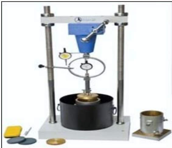
Fig. 2: Swell Pressure Test by Constant Volume Method
