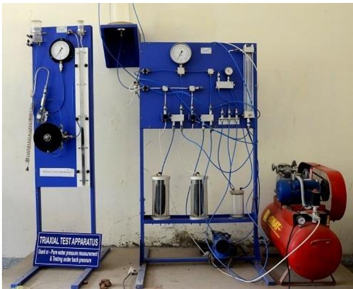
Fig. 2: Triaxial Test Setup
