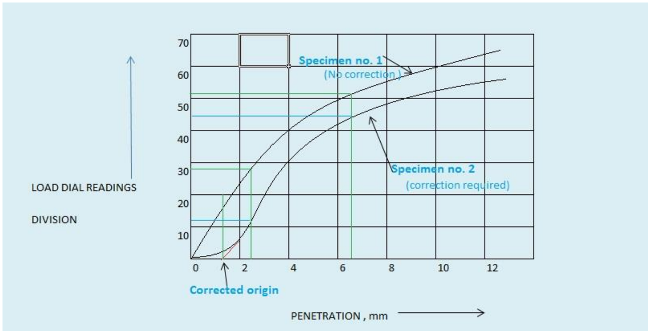
Fig. 4: Plot of Load versus Settlement
