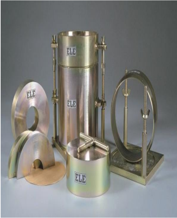
Fig. 2: CBR Mould with Base Plate, Stay Rod and Wing Nut
