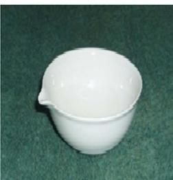
**Fig. 5: Evaporating Dish**
