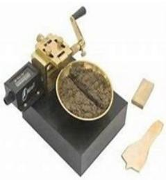
**Fig. 2: Mechanical Liquid Limit Device**
