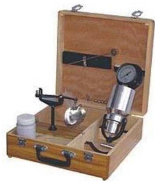
Fig. 1: Setup for Rapid Moisture content Determination
